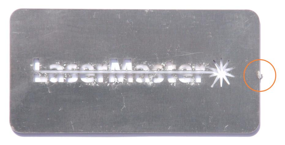
YOU WILL GET A SMALL TAG ON THE OUTSIDE EDGE OF ALL LASER CUT PARTS - IT IS LIKE A SMALL PIP
